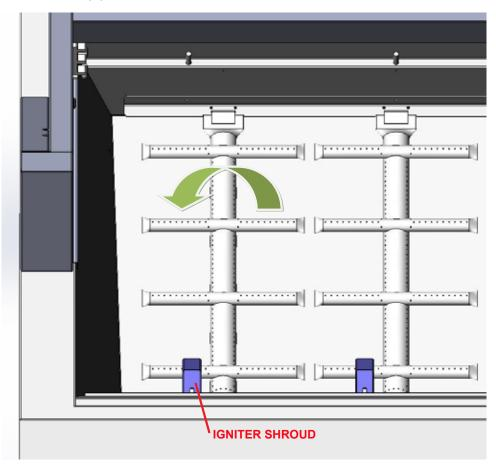
2. You will also need to remove the igniter shroud for the burner you are changing out. Remove both screws shown to reveal the ceramic igniter. Be careful not to damage the ceramic material, it can snap off during reassembly.
