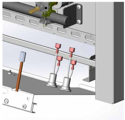
2. Before removing the main burner orifices, take a visual note as to how far the orifice is installed onto the valve body. The orifices are removed with a 1/2'' deep socket wrench. Use even pressure to break loose the old orifice and remove from the valve.
