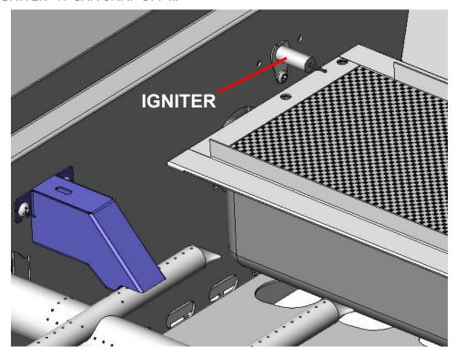
3. With the burner fully inserted, align the hole in the rear bracket with the tiny dimple in the rear firebox wall. If your grill has no dimple, visually align the burner while maintaining the 1.25" vertical distance as shown below. Use a power drill with 5/16" socket to install the self-drilling screw into the rear wall of the firebox. This will secure the sear burner in place. Go slowly - do not strip the threads or the new hole. Replace the metal cover and mesh screen you removed in step 1.
